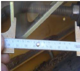
3-inch threaded gap
